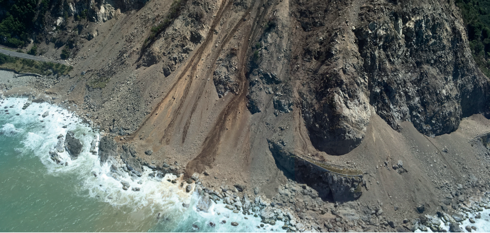
Figure 4: SH1 access along the South Island coast severed by large landslides following the 2016 Kaikoura Earthquake. Similar landslides of this magnitude are expected to occur in Wellington should a major earthquake occur in the region. (Source: Walter Rushbrook / Aurecon)
