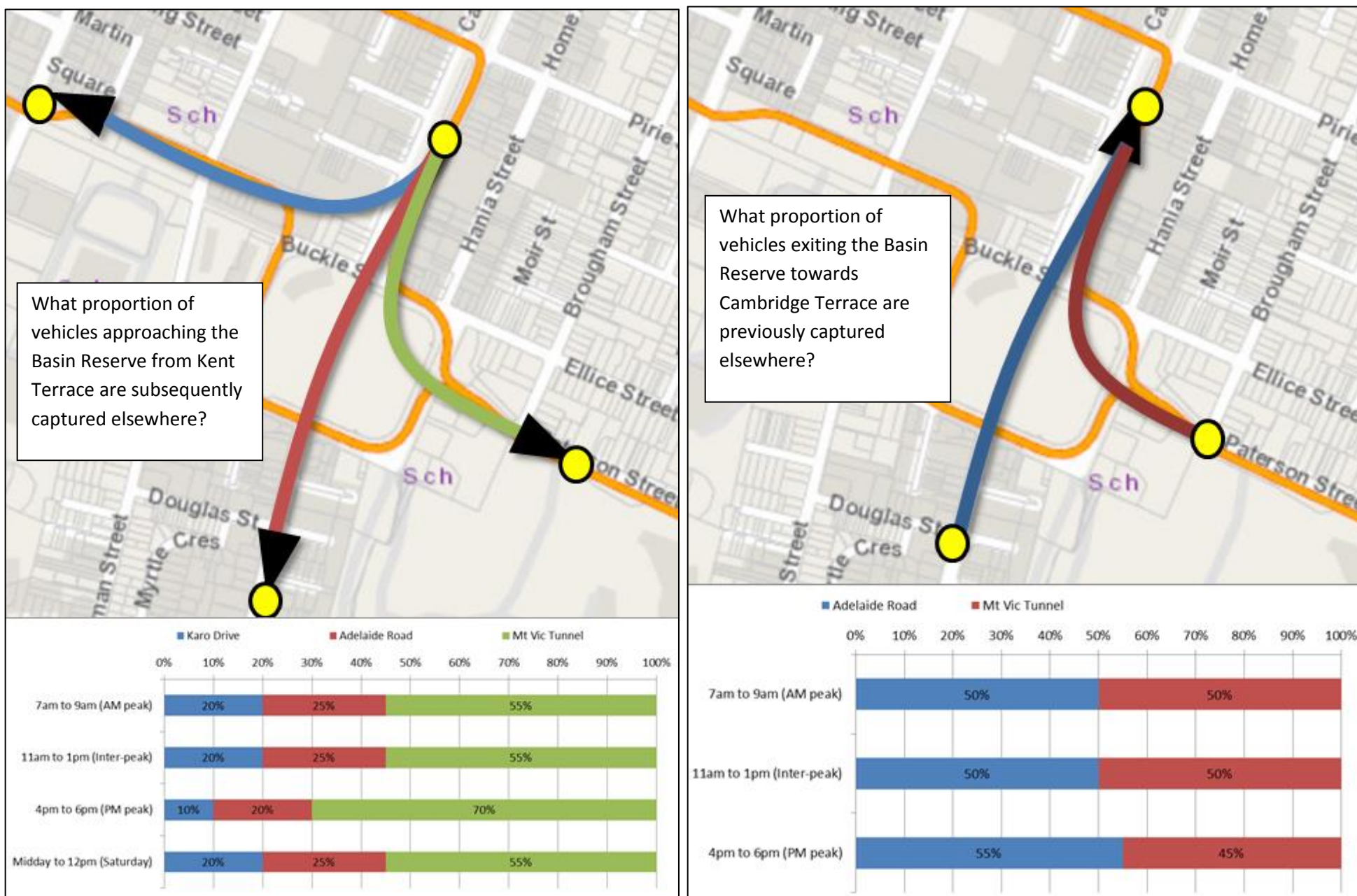
Figure 79 ANPR turning proportions at the Basin Reserve – Kent / Cambridge Terrace
