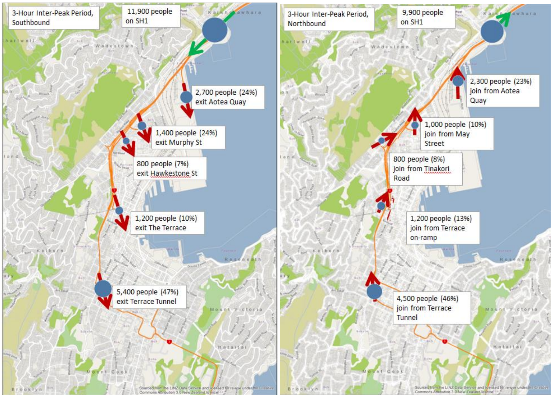
Figure 72 Inter-peak (11am to 2pm) – exit points for traffic on SH1 southbound approaching Aotea Quay (left) and joining points for traffic on SH1 northbound past Aotea Quay (right)
