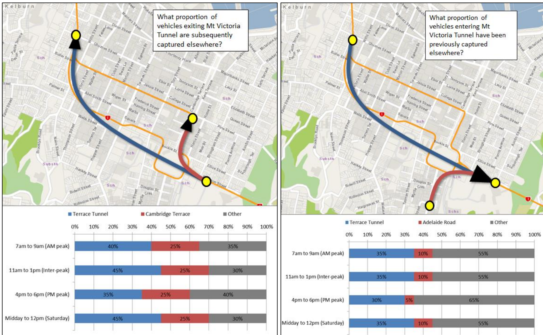
Figure 76 Mt Victoria Tunnel – tracking of vehicles by Automated Number Plate Recognition (ANPR) exiting Mt Victoria Tunnel (left) and entering Mt Victoria Tunnel (right)
